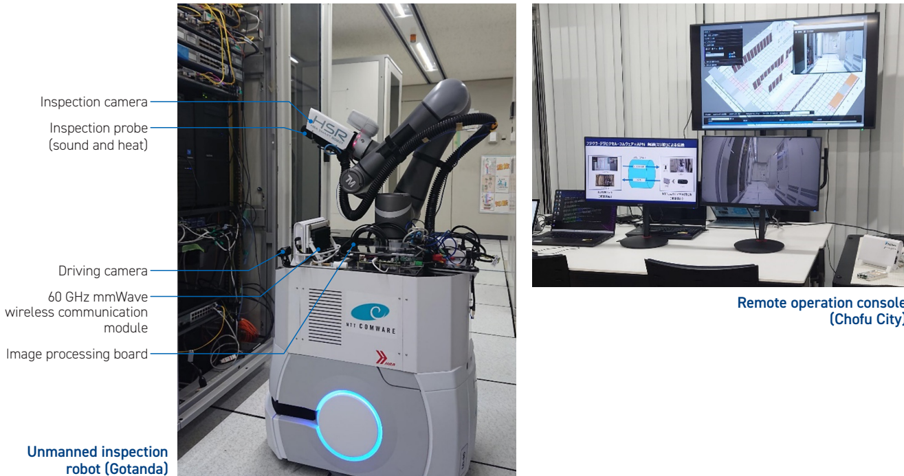
■ Trial of remote robot operation via low-latency video transmission using 60GHz mmWave wireless
